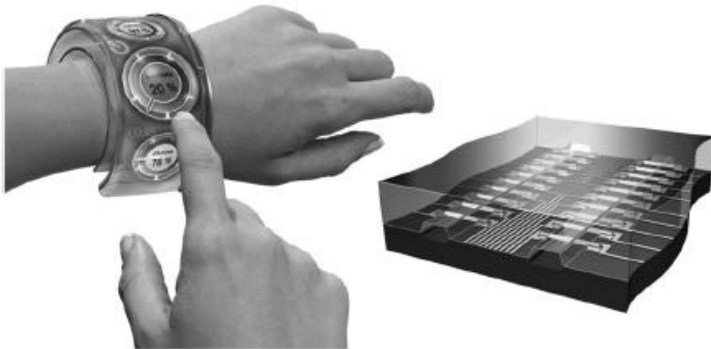
Fig. 5 The Nokia Morph concept mobile device ( http://www.nokia.com/A4852062 ) showing its biosensor capability based on nanowire sensors and a sample output of key physiological markers for sporting performance.
